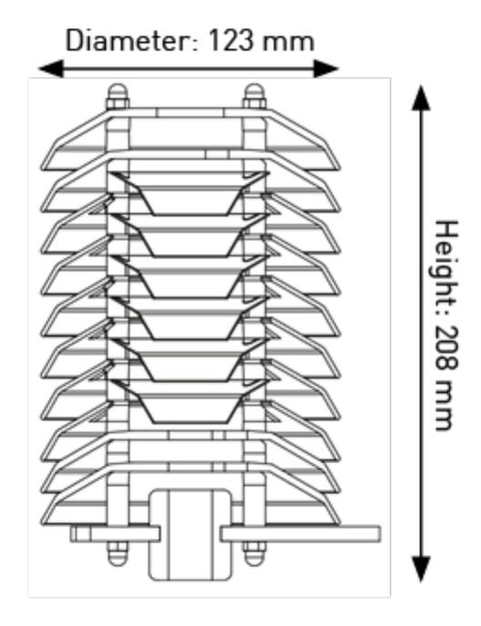
Overall height including bracket: 300 mm Weight: 1.01 kg
