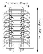
Overall height including bracket: 300 mm Weight: 1.01 kg
