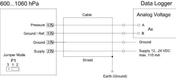
HT0 Jumper P1: 1-2 / PS2 Slope: 92 Offset: 600
