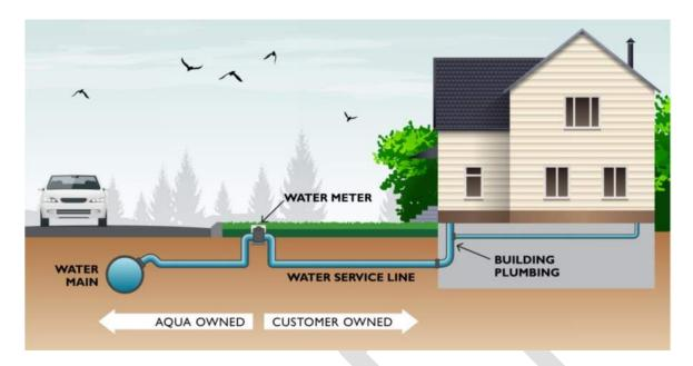
Figure 1-2: Diagram of a Water Service Line
